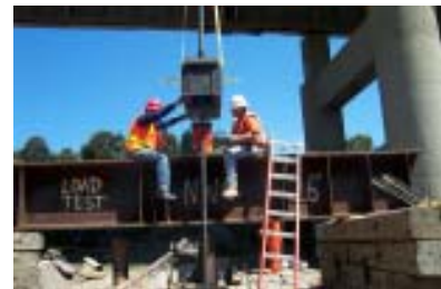
Test Set up for 400 kip Tension Test
